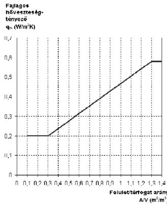
Specific net heating energy demand W/m<sup>3</sup>K vs surface to volume ratio
